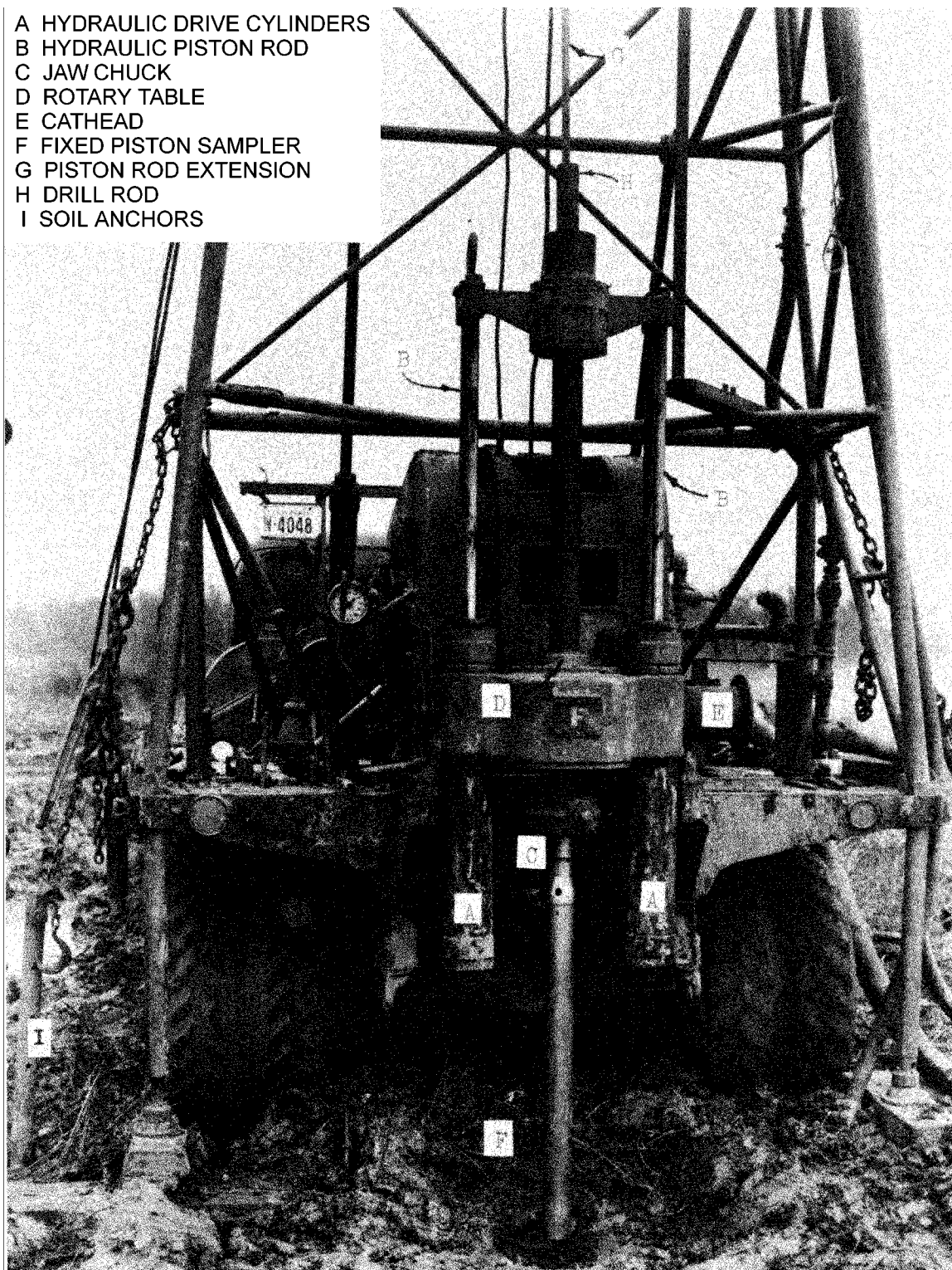
Figure 3-2. Photograph of a truck-mounted rotary drill rig with specific features of the drill rig identified
